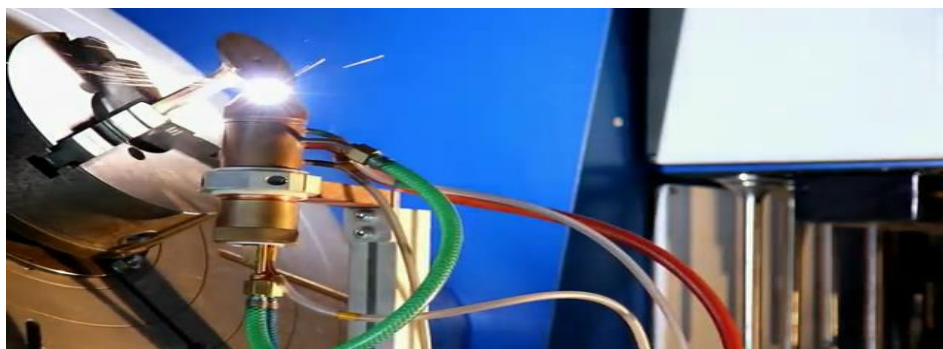
2 – rasm. Klapan tarelkasini plazmatron yordamida payvandlab qoplash jarayoni
