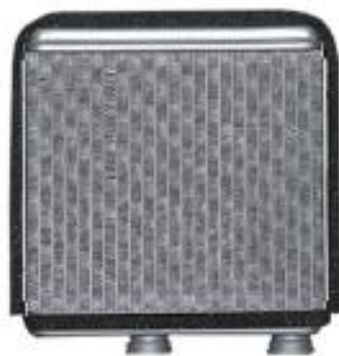
1-rasm. Spark avtomobilining isitish pechi
