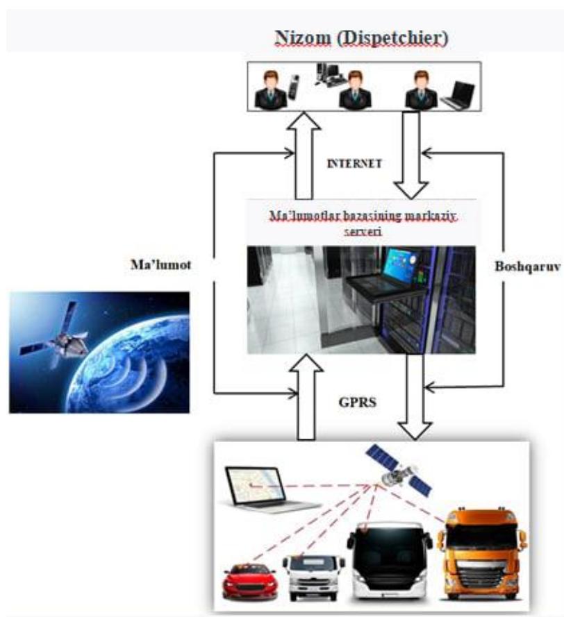
2 - rasm. Transport vositalarining harakailanish parametrlari haqida navbatchi nozim (dispetcher) ga axborot yuborish sxemasi.
