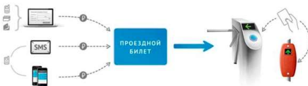
1- rasm Transport kartalarining ishlash sxemasi
